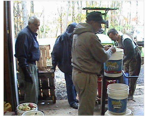
After the apples are washed they are taken from the buckets and placed in the hopper where they made into pulp to be pressed to get the juice.
