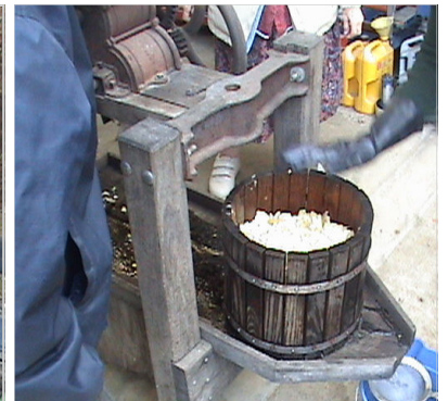
Here you see the apples ready to be pressed after they are grinded.
